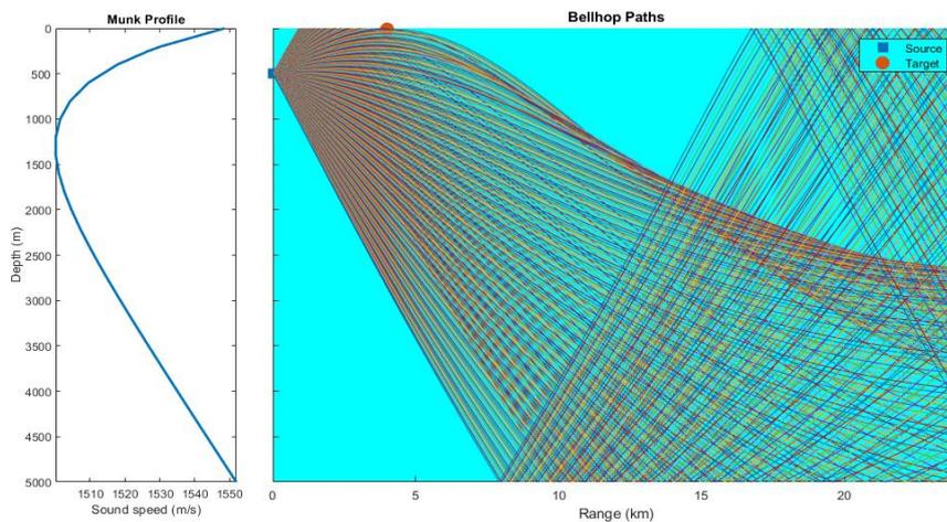
**Fig. 4.** Bellhop Ray Trace for Case 3
