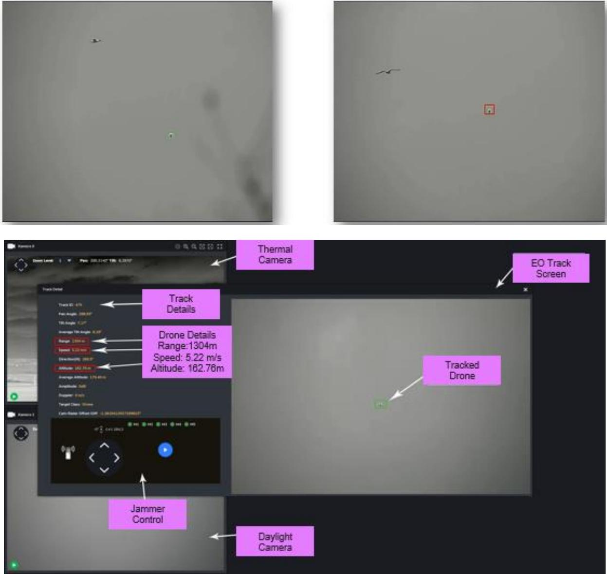
**Figure-4: KAPAN Anti-Drone System**
