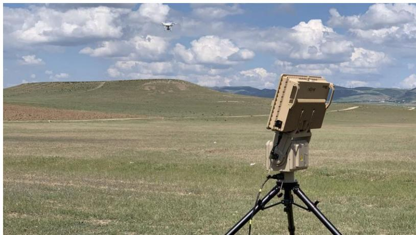
**Figure-3:** Retinar FAR-AD Drone Detection Radar
